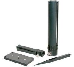
The **Man-pack Antenna** provides 8dB of gain and allows the communications operator to hold the antenna, place it securely in the ground or attach it to a vehicle with powerful magnets. The antenna provides a frequency range between 243 to 318 MHz in SATCOM mode and 225 to 400 MHz for UHF LOS mode. **Each antenna comes with a hardened ground spike, magnetic mount, standard kit bag, and a choice of either pistol or straight grip handle**. There is also a optional tactical holster.
